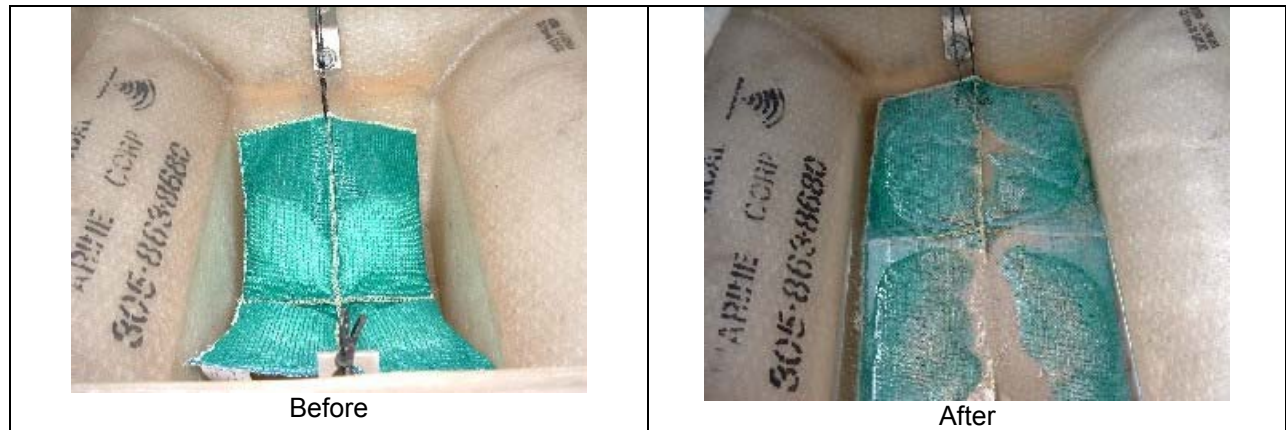
Figure 24. Photographs of Hydro-Cartridge™ During the Continuous Dose Plus Sediment Experiment.
