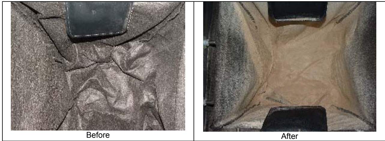
Figure 26. Photographs of Drain Pac™ During the Continuous Dose Plus Sediment Experiment.
