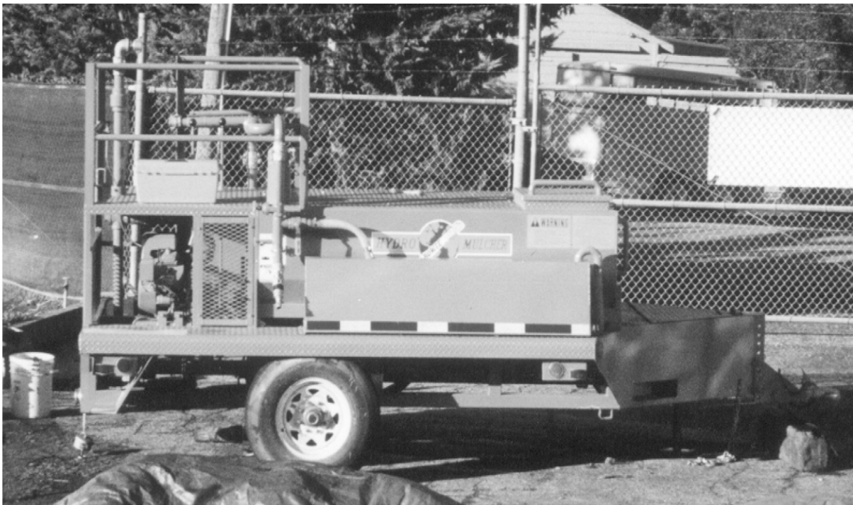
Figure 1. 600-gallon hydromulcher used to apply mulch materials.
